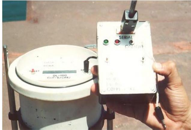
(Figure-4 DIGILEVEL: Control Unit with Data collector)
