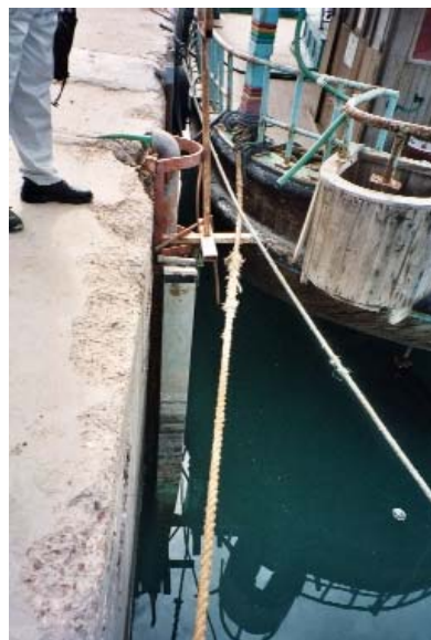
Figure 3 and 4. Valeport Model 710 installed at the fishing village Nakhl-e Taghi.
