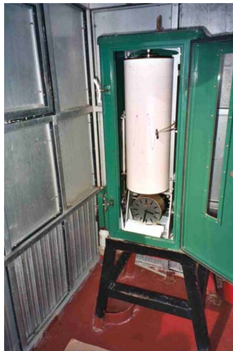
Figure 8. Float gauge manufactured by the Ott company.
