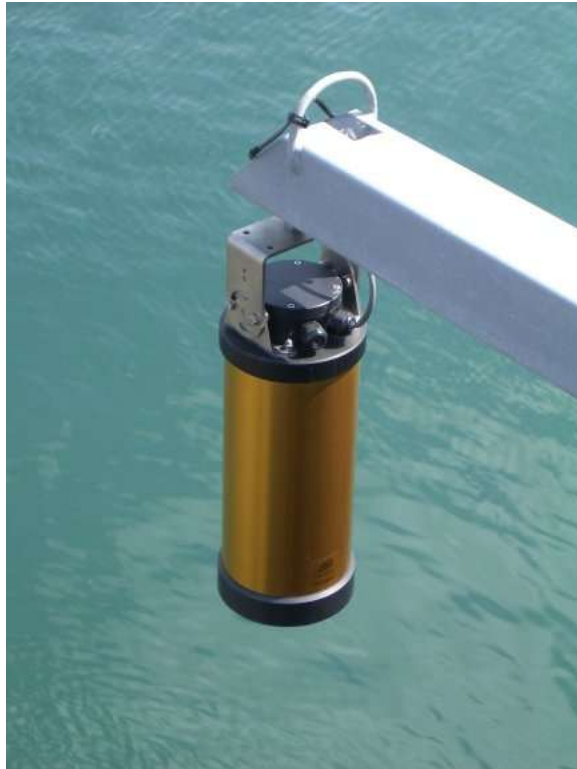
Illustration 6- OTT Kalesto supported from steel arm
