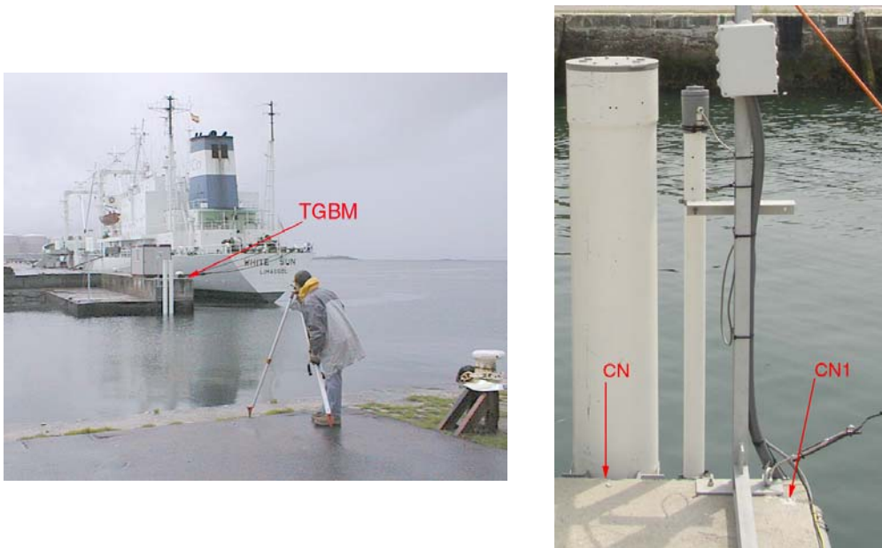
Figure 13 Levelling of the Tide Gauge Bench Mark (TGBM) and zoom in the auxiliary marks.
