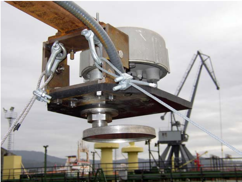
Figure 5 Horn antenna of the RADAC tide gauge.
