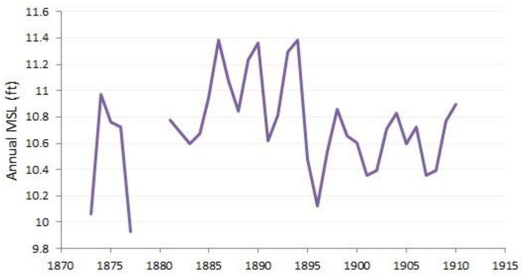
Figure 16: Annual Mean River Level from Kidderpore showing the suspected datum step around 1894, (compared with the earlier and later data)
