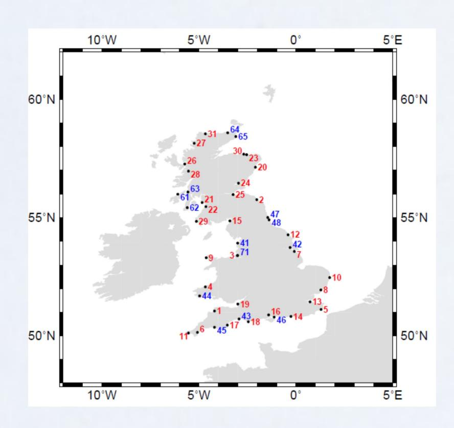
In 1859-60 the Ordnance Survey made sea level measurements for a fortnight at 31 locations shown in red (other stations of interest with data at about the same time are in blue). MSL was measured to Ordnance Datum Liverpool (ODL) at this time.
