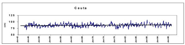
The slope of the linear fit y=ax+b is 0.61 mm/year.
