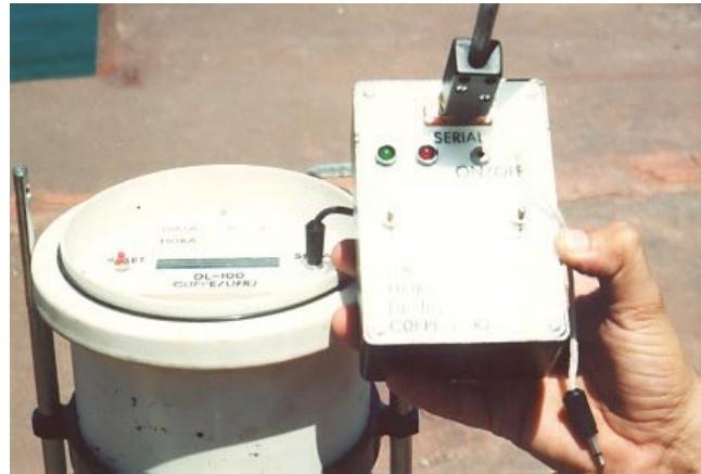
(Figure-4 DIGILEVEL: Control Unit with Data collector)
