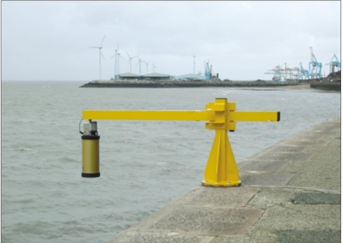
Figure 2: The OTT Kalesto gauge installed at Gladstone Dock, Liverpool
