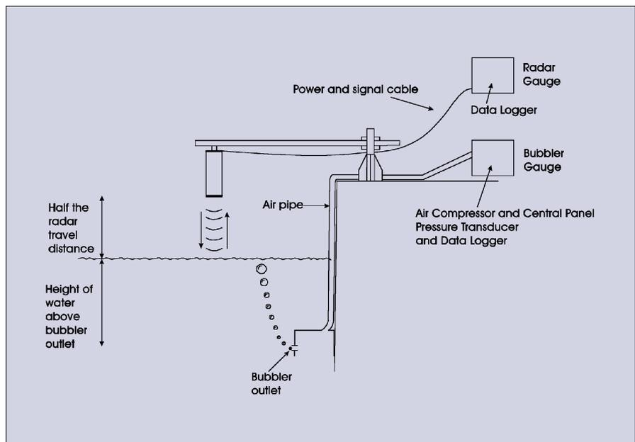
Figure 1: A schematic description of the radar and bubbler gauge systems at Liverpool
