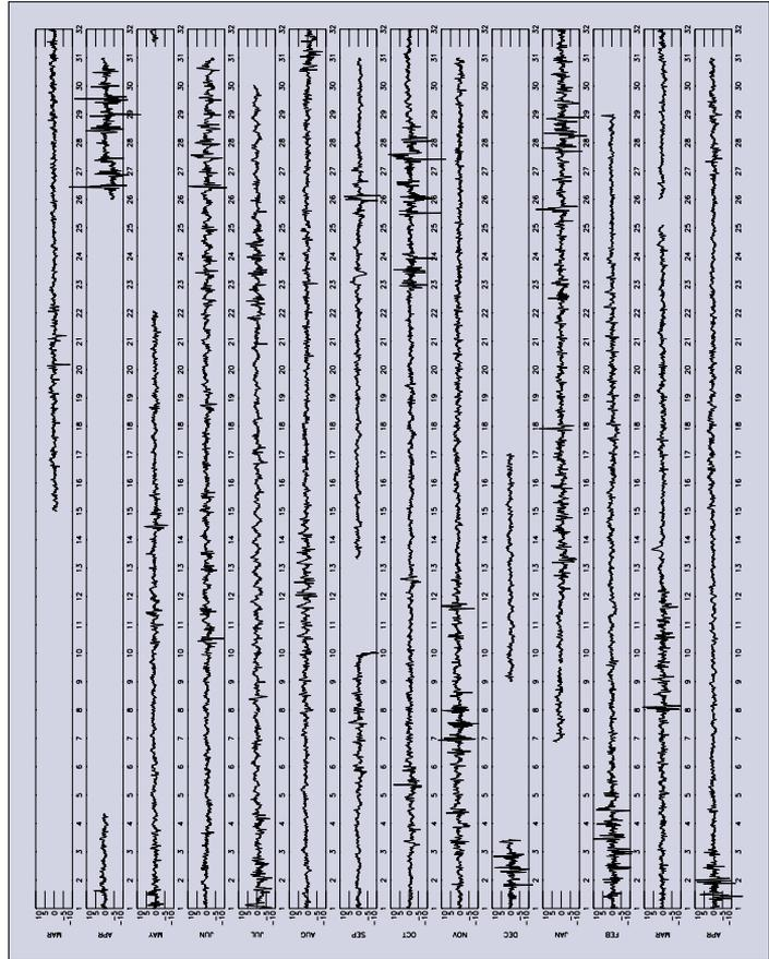
Figure 4: Time series of radar minus bubbler residual-differences. Vertical scale  $\pm 10$  cm
